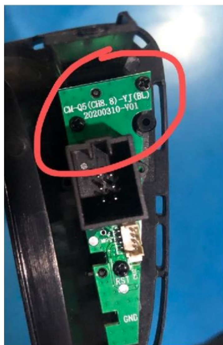
PCB with BL is for Pass. Airbag Off indicator equipped vehicle (e.g. the US)
