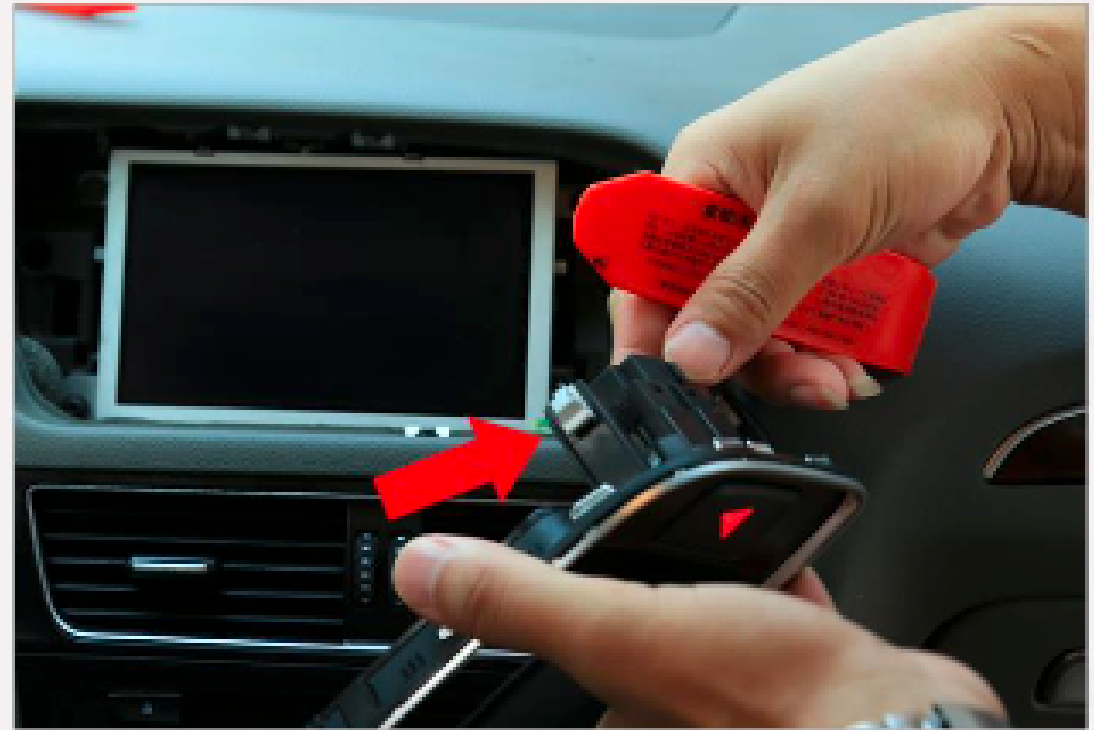
2. Unplug the emergency hazard button connector and remove the screen fascia. Also remove the factory original screen unscrewing 4 T20 screws.
