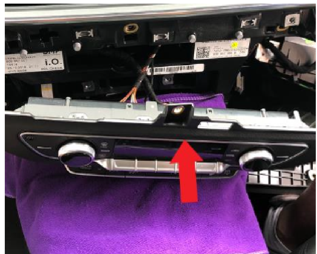
12. Unscrew the upper screw holding the center dash climate control panel trim and carefully remove the trim.
