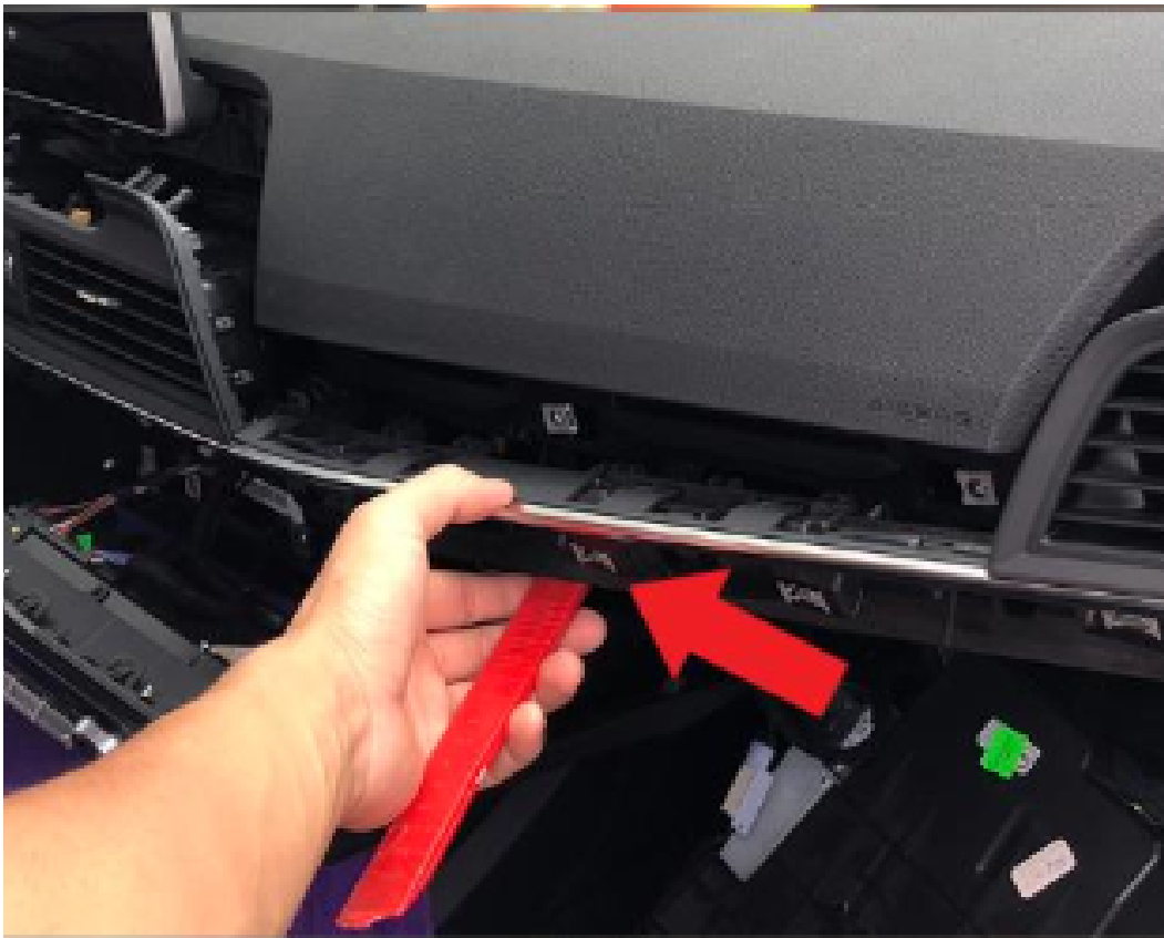
13. Pry out the center dash air vent frame assembly.
