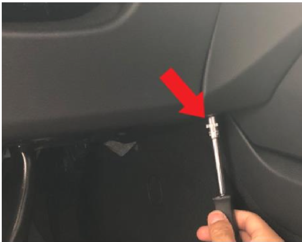
7. Remove the screws located on the bottom of the glove box compartment.
