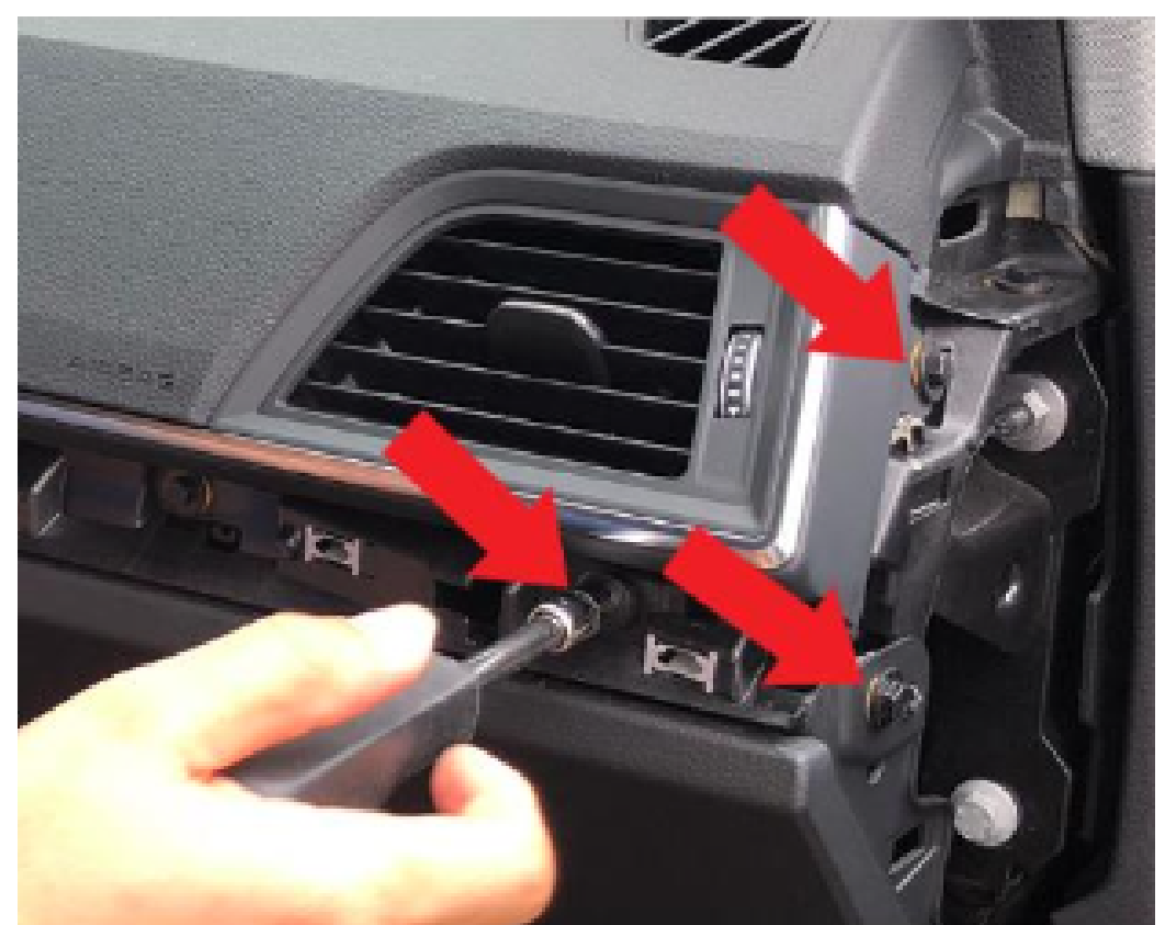
4. Remove the horizontal dash trim by prying from the bottom and pulling outward.
