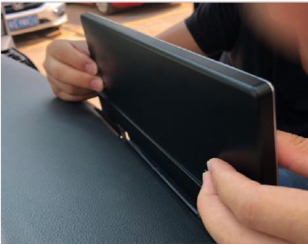
19. Press the two locking points behind the new screen.
