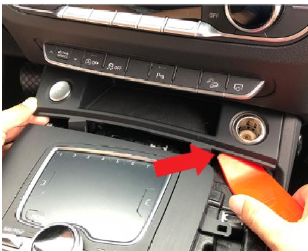
11. Remove the start button & cigarette socket assembly by prying from the bottom.
