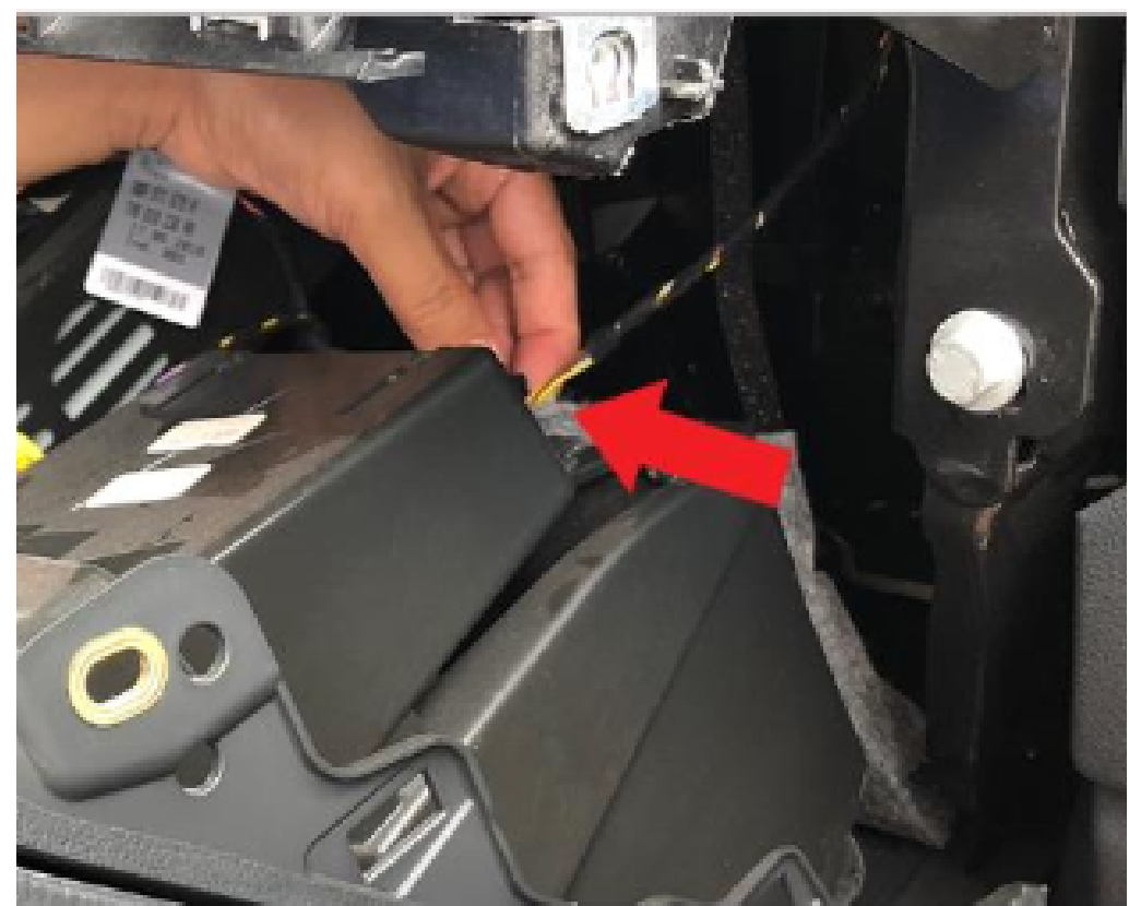
8. Unplug removable connectors from the glove box.
