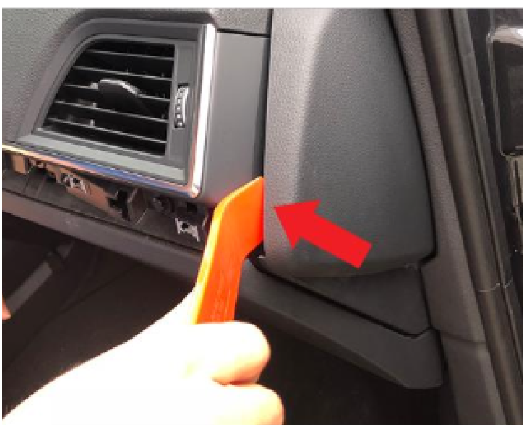
5. Remove the passenger side fuse panel cover.
