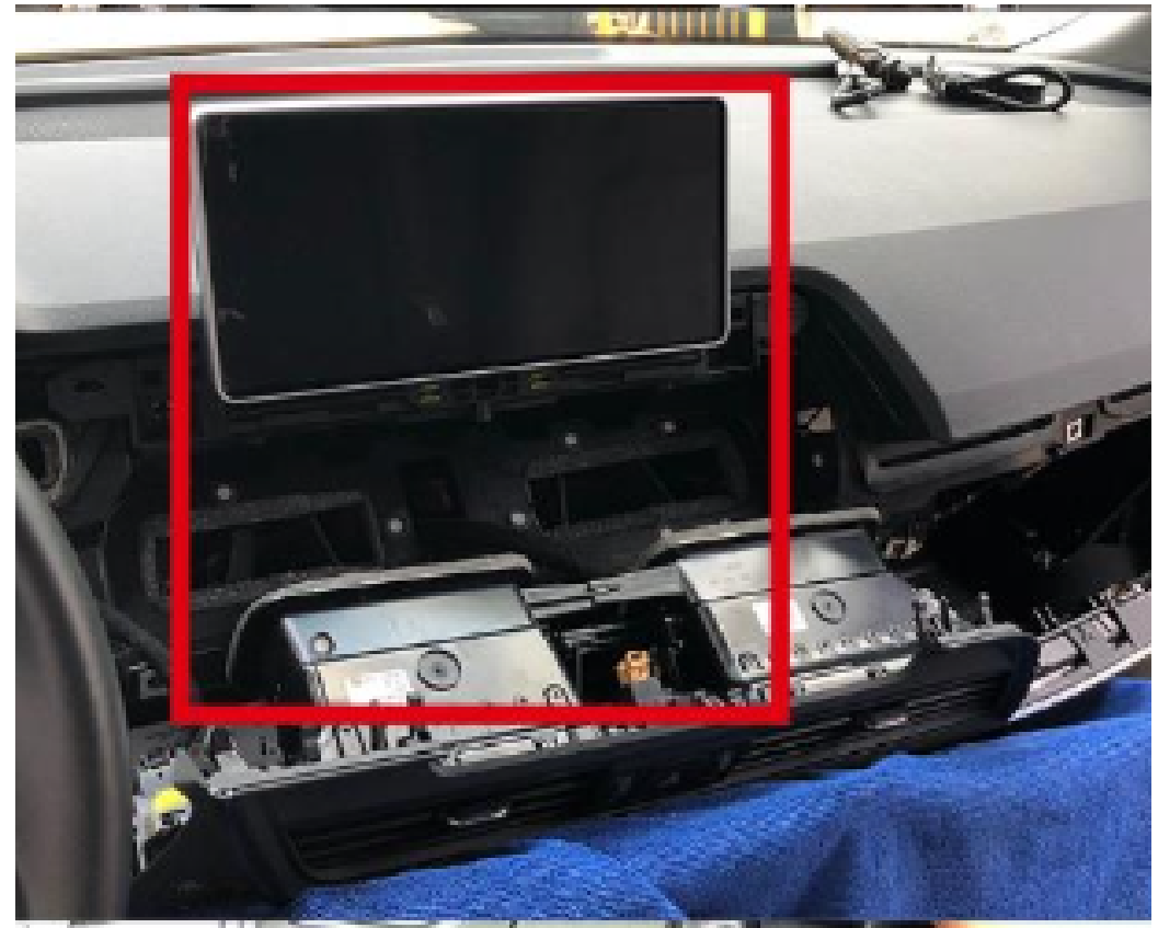
14. Place a large towel under the removed frame and disconnect necessary connectors.
