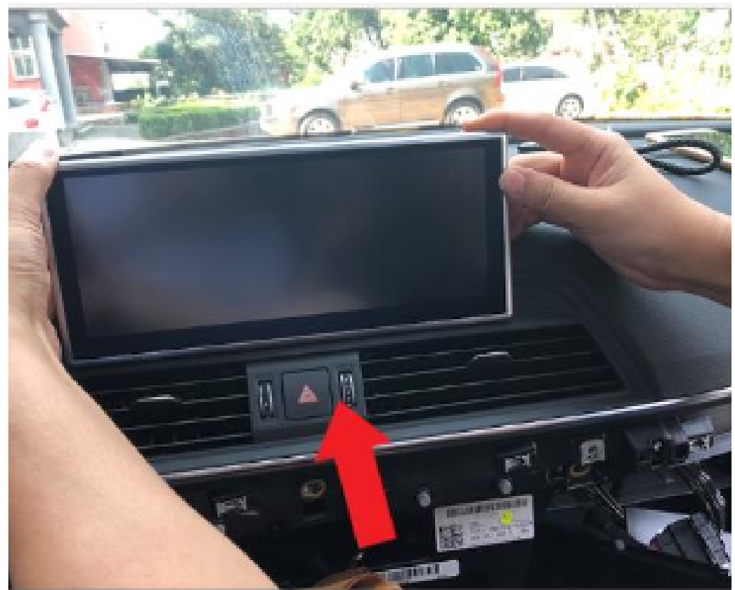
20. Carefully lift up the screen. Do not try to remove the screen completely as it is not designed to be removable.
