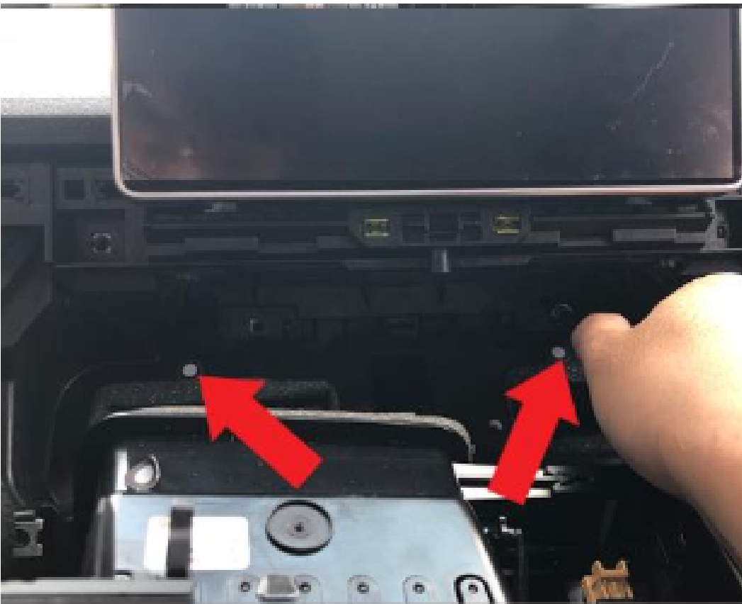
13. Pry out the center dash air vent frame assembly.
