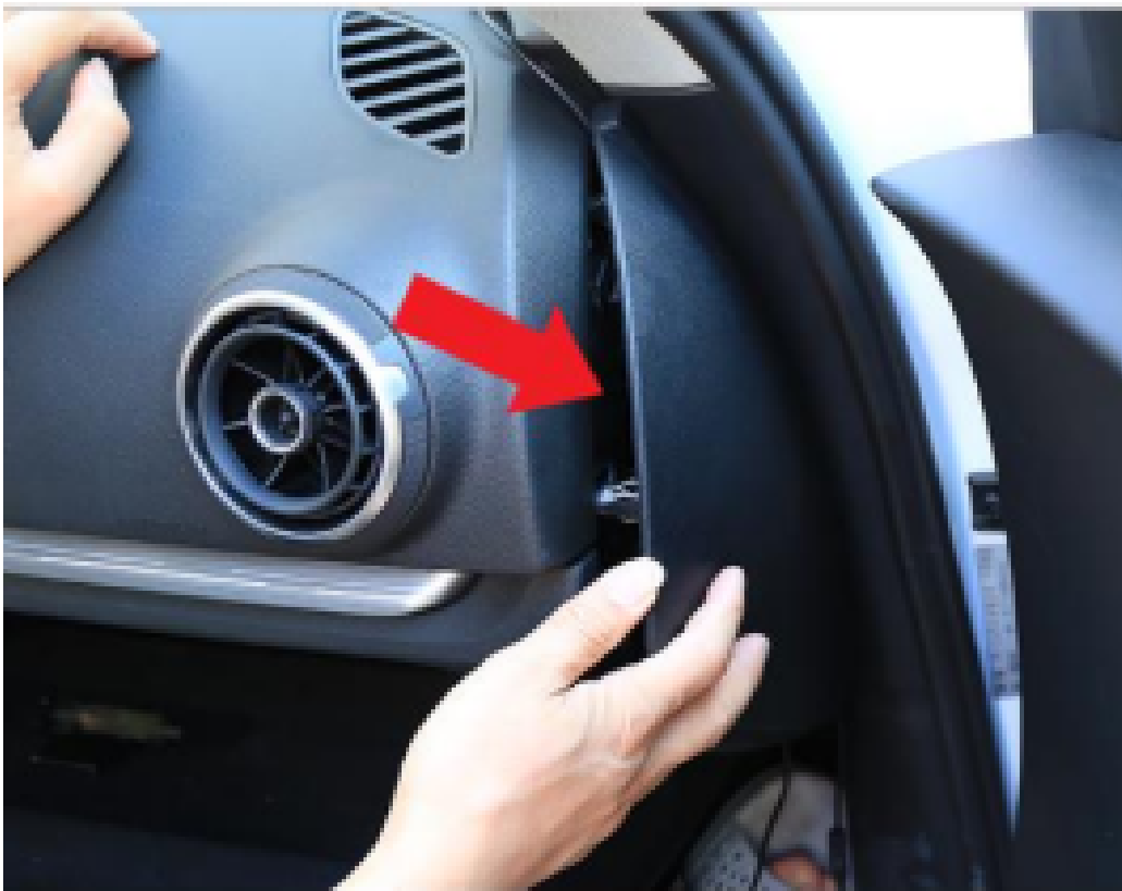
7. Remove the passenger side fuse panel cover.
