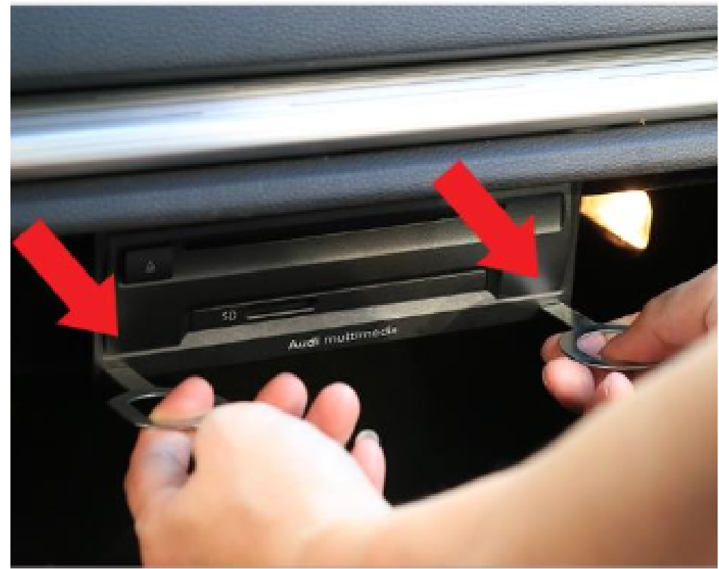
8. Remove the MMI head unit inside the glove box using VAG Radio removal keys.
