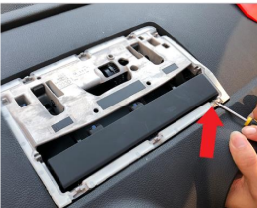
5. Using a hook, carefully lift up the screen mechanism assembly.
