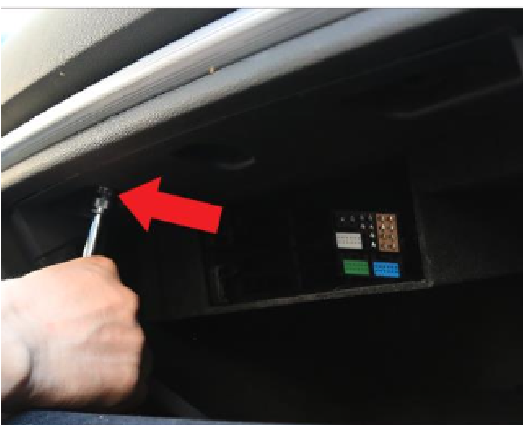
9. After unplugging every connector behind the MMI unit, there is one 8 mm hex screw to be removed. Unscrew it for further installation.
