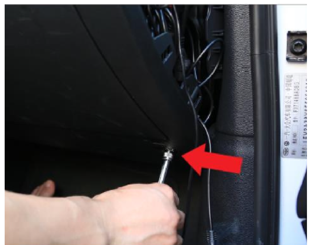
12. Remove the bottom screws of the glove box.
