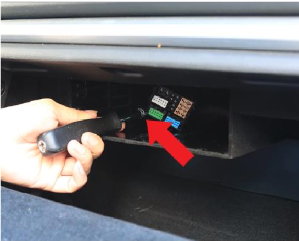
9. After unplugging every connector behind the MMI unit, there is one 8 mm hex screw to be removed. Unscrew it for further installation.
