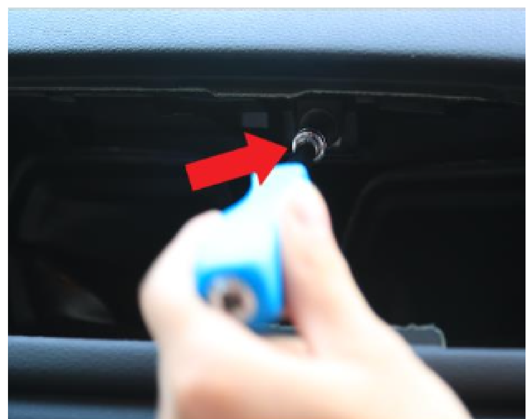
6. Unscrew the 8mm hex screw holding the screen.
