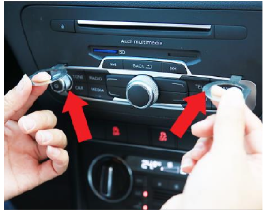
2. Use VAG Radio removal keys to remove the Radio/MMI head unit.
