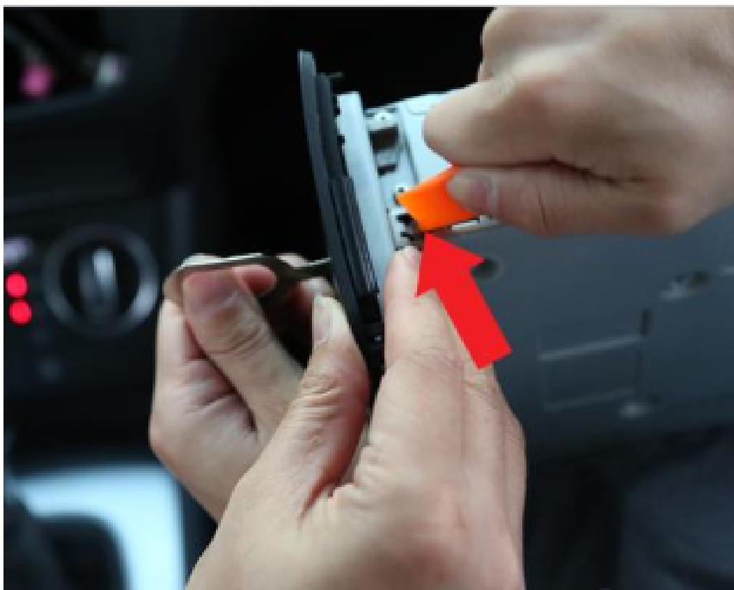
3. To remove the VAG key, push it in and upward, then pull the key out while holding the locking mechanism.
