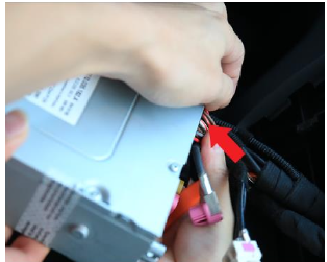
4. Unplug all the connectors behind the radio/MMI.
